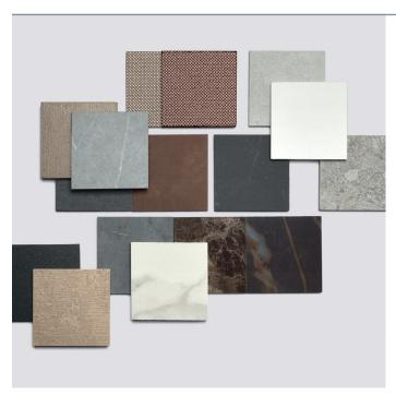
**Gres** is the most durable ceramic of all. It is particularly suitable for covering floors and walls in highly humid or large passageways. Very easy to clean, it is a compact and robust material as well as being flame retardant and not emitting organic compounds of any kind. It is well resistant to scratches and stains so it also lends itself to covering the bathroom floor or as a cover for doors and furniture. For cleaning it is possible to use warm water and neutral detergents.
