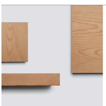
**Solid wood** is obtained from the centre of the tree, that is, from the most resistant and solid part of the trunk. It is used to create durable furniture of excellent quality while also being warm and pleasant to the touch. Solid wood is a unique, precious and authentic material, with a hand-barked edge, externally finished with a natural varnish. Normal cleaning can be performed with a damp non-abrasive cloth, while in case of stains a neutral detergent diluted in water is recommended.
